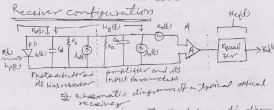
three stages namely, a photodetector, an amplifier and an equalizer. The P.D. can be either an APD with mean gain  $M$  or a PIN P.D. for which  $M=1$ . The P.D. has a quantum efficiency  $\eta$  and a cap. Ed. The detector bias resistor has a resistance  $R_b$  which generates a thermal noise current  $i_b(t)$ .
